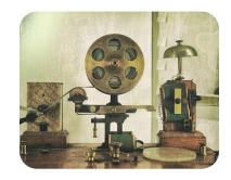
The telegraph was a system for transmitting messages along a wire by making and breaking an electrical connection.
